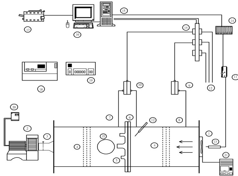
Fig. 2 Sketch of AMCA test chamber and instrument setup
