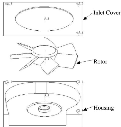
Fig. 1 The structures and components of a typical cooling fan for notebook computer
