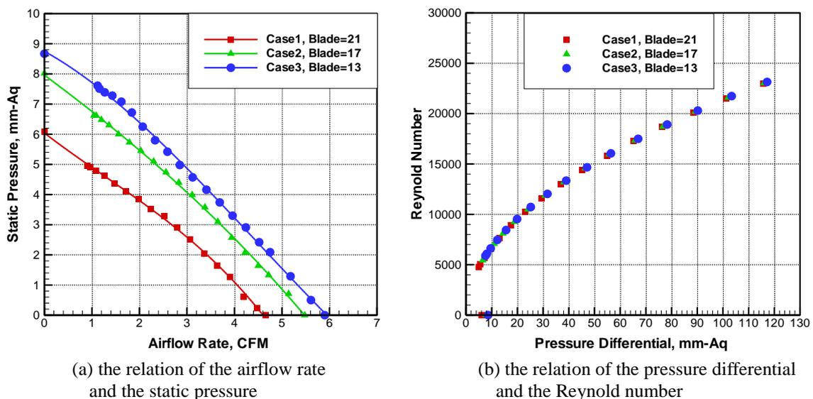
Fig. 7 The performance curves for different case of centrifugal cooling fan
