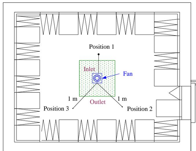
Fig. 4 Schematics for the positions of noise measurement
