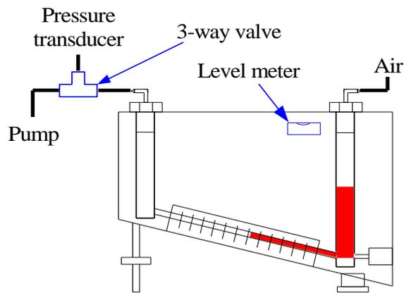
Fig. 3 The pressure calibration system
